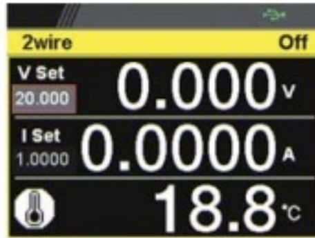
White: Temperature Control on with GTL-205A Connected
