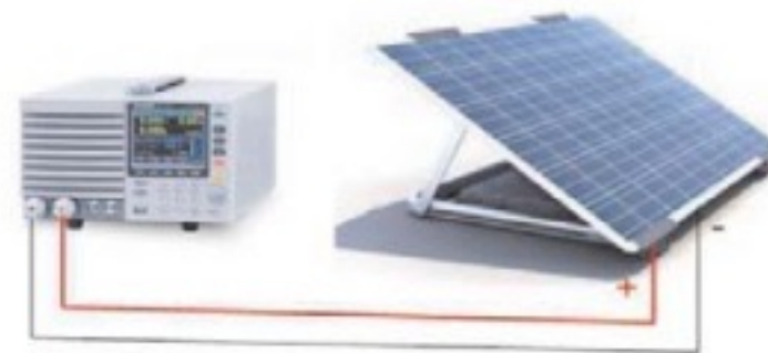
Connections Between PEL-3041 and Solar Panel
