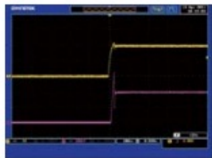
The Inrush Current and Surge Voltage occur at LED Forward Voltage ( V_f ) Under C.V Priority
