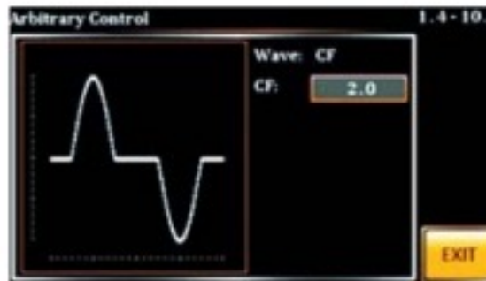
Crest Factor Waveform Simulate Rectified Filter Current Waveform By Capacitor Input
