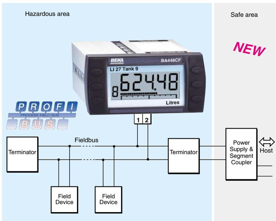
The **BA448CF-P PROFIBUS Indicator** is an intrinsically safe instrument that can display up to eight fieldbus process variables within a hazardous area. A numeric annunciator on the left hand side of the screen shows which variable is being displayed. This version of the indicator supports PROFIBUS PA protocol; for FOUNDATION™ fieldbus systems an alternative version is available – please see BA448CF-F FOUNDATION™ fieldbus datasheet.
