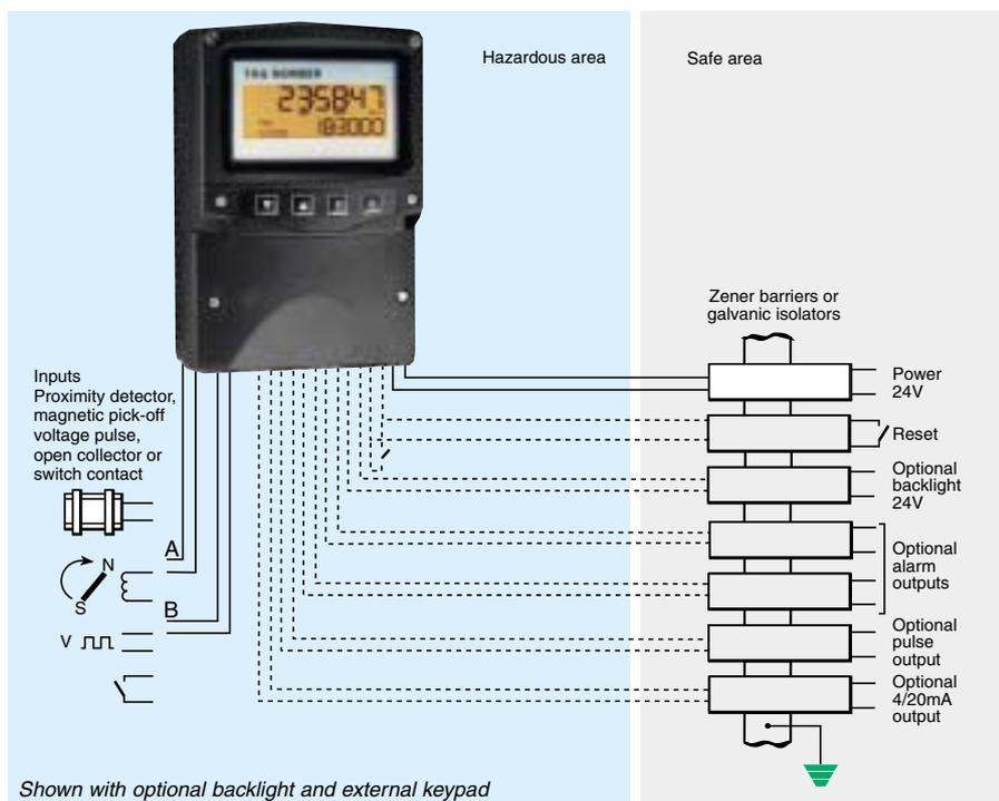
The **BA364D** is an intrinsically safe multi-function instrument which may be programmed to perform a host of counting and timing functions. Easy to use menus allow the instrument to be configured as a counter, timer, tachometer or as a clock. Both of the inputs will operate from 2-wire proximity detectors, switch contacts, magnetic pick-offs, open collectors or voltage pulses. Optional alarm/control outputs further extend the many applications.
