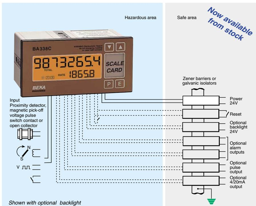
The **BA338C** is an externally powered, intrinsically safe rate totaliser with separate rate and total displays which will operate from a switch contact, voltage pulse, magnetic pick-off, open collector or a proximity detector input. A novel adaptive measuring technique plus an adjustable digital filter ensure that optimum rate display stability and step response can be achieved over a wide input frequency range.
