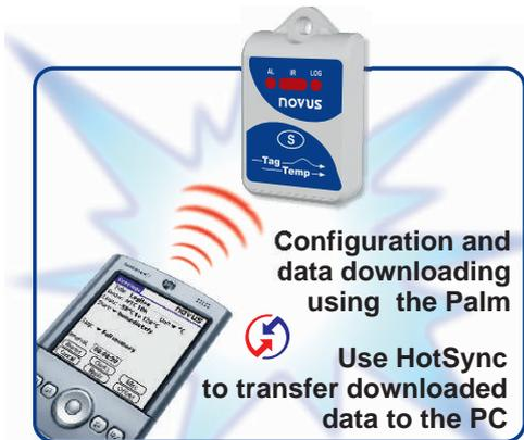
Configuring and downloading data with Palm OS compatible devices by means of the Infrared interface is easy and convenient. The data can be transferred to a PC through the **HotSync** synchronizer.
