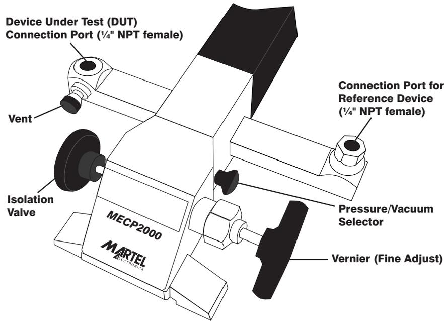
1. Connect the pressure reference (calibrator or digital gauge) to the right side reference device connection port. Be sure to use Teflon tape to seal the threads. A BSPP adapter is provided if needed.
