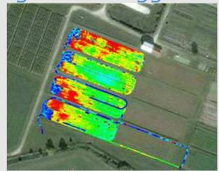
GPS-signal acquisition is a further function in Delphin's data logger. Positional fixing of **mobile applications via GPS signals** has proved to be highly popular. GPS signals are received via GPS sensors and transmitted to the data logger via a serial cable. The GPS coordinates are then processed as measurement channels. Measurement data is then correlated to a specific location.
