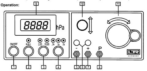
Pressure output P should be connected with 6 mm tube at a low or negative pressure using a T-piece to the pressure to be measured as well as to the pressure intput "+" resp. "-" for vacuum. For large displacement volumes the measuring pressure is set to course using the pump [10]. Fine setting is made with knob [11].
