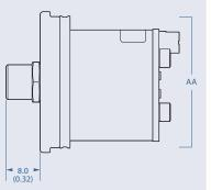
M8 connector cable or terminal block. Works with 2-, 3-, 4-wire RTDs.
