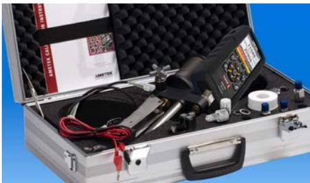
Combine the APMi pressure modules with the HPC50 calibrator and any of our pump systems. From small pneumatic hand pumps to a precision, hydraulic pressure comparator capable of generating up to 15,000 psi (1000 bar), we have the perfect kit for your application.
