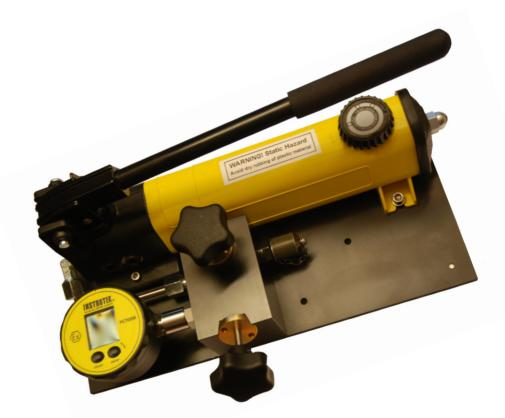
**High accuracy and stability** - is achieved by use of a piezoresistive transducer with a built-in temperature compensation. Unlike some other pressure calibrators, accuracy is maintained when decreasing pressure which makes the unit ideal for verification of hysteresis. All units are calibrated in positive as well as in negative direction.
