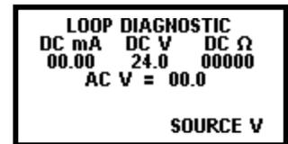
In all loop diagnostic modes, AC voltage is displayed. If more than 2 VAC is present on the Model 532's terminals, the display is highlighted to alert the user of a potential problem.
