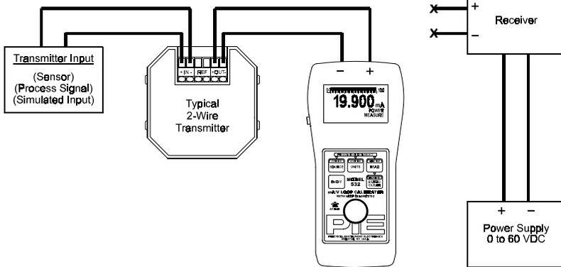
The Model 532 provides power to the process loop while displaying output current. Use this mode to test a transmitter's ability to control loop current. Current limiting above 24.000 mA is indicated by a flashing "CURRENT LIMITED" display.
