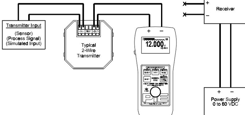
The Model 532 sources 0.000-24.000 volts. This is useful for powering transmitters and receiver equipment. Use the EZ-Dial™ Knob and EZ-Check™ Switch to adjust output voltage. The display flashes "LOW Ω" when the output is overloaded.
