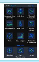
The onboard applications provide a useful selection of features including HART communicator, high static differential pressure mode, pressure leak test, safety valve test, analog transmitter calibration, unit converter, thermal calculator, and snapshots to name a few.
