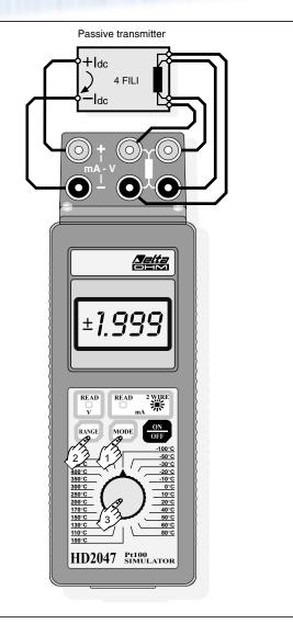
Fig. 3 Verification of a passive transmitter with Pt100 input
