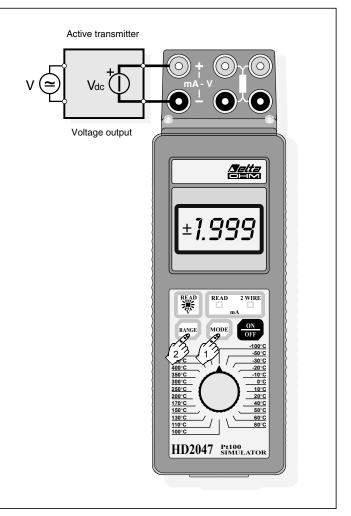
Fig. 1 Continuous voltage measurement
