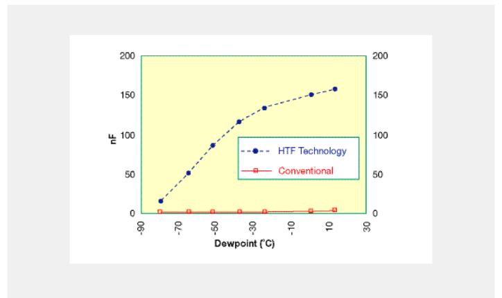
Hyper Thin Film vs. Conventional  $AI_2O_3$  Sensor. Change of Capacitance with Dew Point
