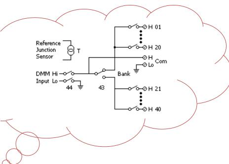
DAQ-903 can switch 40 single-wire inputs per module. It can be used for common-low applications such as battery testing, component characterization and desktop testing. The low-voltage connection is isolated from ground and can be floated up to 300 V.
