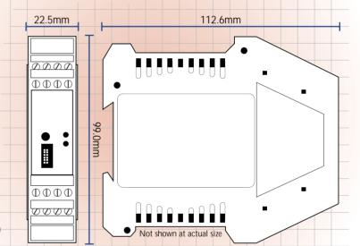
Note: Depth 114.5mm when mounted on Din Rail TS35 / TS35D
