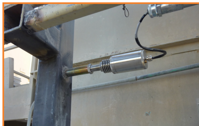
Mass flow measurement of dry sand
