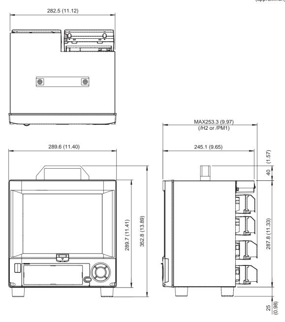
Note: If not specified, the tolerance is  $\pm 3\%$ . However, for dimentions less than 10mm, the tolerance is  $\pm 0.3$ mm.
