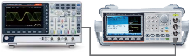
Direct Waveform Reconstruction from the DSO
