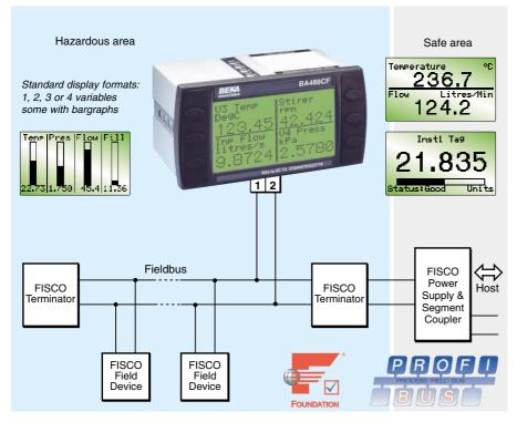
The BA488CF Fieldbus Display is an intrinsically safe instrument that can display up to eight fieldbus process variables. Nine selectable standard screen formats contain one, two, three or four variables, with units of measurement, tag descriptions and bargraphs on some screens. The use of standard screens simplifies commissioning, but if required dedicated screens tailored to an individual application can be constructed.
