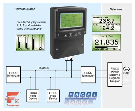
The BA484DF Fieldbus Display is an intrinsically safe instrument that can display up to eight fieldbus process variables. Nine selectable standard screen formats contain one, two, three or four variables, with units of measurement, tag descriptions and bargraphs on some screens. The use of standard screens simplifies commissioning, but if required dedicated screens tailored to an individual application can be constructed.
