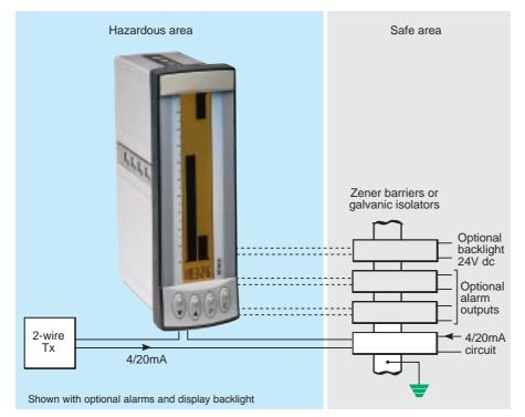
The BA326C is a new combined analogue and digital indicator which replaces the BA326B. It offers enhanced features and improved visibility in a shorter enclosure. Like its predecessor, the BA326C displays the current flowing in a 4/20mA loop on both a 100 segment bargraph and in accurate engineering units on a digital display. The instrument is loop powered but only introduces a 1V drop allowing it to be installed in series with almost any 4/20mA loop.
