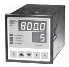
The Nokeval multipoint indicator 538-5 is designed for applications, where display, output signals and alarms are desired for several measurements simultaneaously. Each input channel can be individually configured for various input signals. For example, the first channel may accept thermocouple input, the second one Pt100, the third channel 4-20 mA, and so forth. Mathematical functions, such as addition, subraction, multiplication or division, can be made between the channels.
