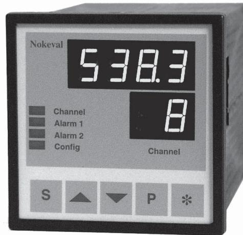
The Nokeval multipoint indicator 538-8 is designed for applications, where display, output signals and alarms are desired simultaneously for several measurements. Each input channel may be configured individually. For example, the first channel can accept thermocouple, the second one Pt100, the third 4...20 mA and etc. The scanning interval of display is adjustable. The 538-8 provides 12 alarms, 2 relay alarms as standard and 10 alarms on an extra card. 538-8 employs 8 analog outputs,
