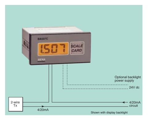
The BA507C is a general purpose panel mounting indicator which displays the current flowing in a 4/20mA loop in meaningful engineering units. The instrument is loop powered, but only introduces a 1V drop allowing it to be used in series with almost any 4/20mA loop. Modular accessories enable only the required features to be selected thus reducing cost while retaining interchangeability between instruments.
