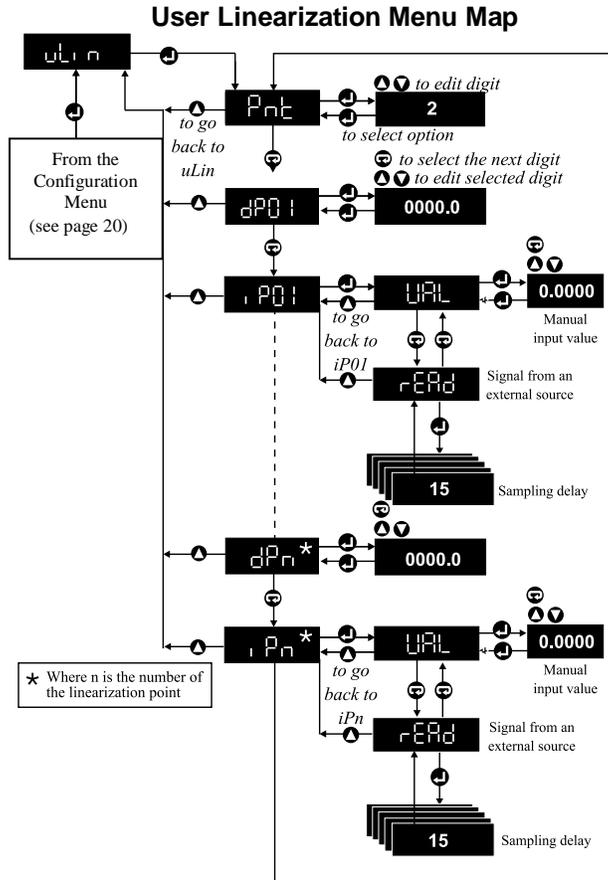
The instrument can automatically linearize most types of thermosensor signals, as long as the **rng** (range) parameter (see **Range** page 22) has been correctly set within the **inPt** (input) menu.
