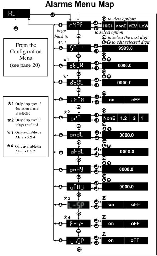
Each alarm can be high or low acting or a deviation alarm. When an alarm occurs:
