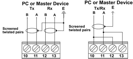
4-Wire & 2-Wire Communications Interface Connections
