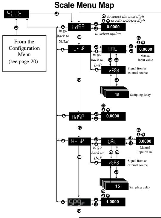
If the scaling is changed via comms, the instrument must be told when to use the new setup by setting Logic Location 12 On.
