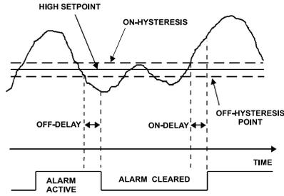
**Effect of Delay and Hysteresis on a High Alarm**
