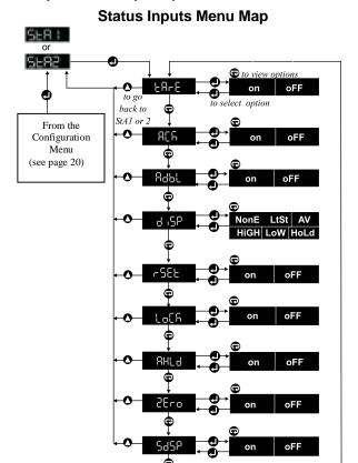
Status Input 1 is activated by connecting Terminal 15 (Status 1) to Terminal 16 (common). Similarly, Status Input 2 is activated by connecting Terminal 14 (Status 2) to Terminal 16 (common). (See **Connections** page 5 and **Connecting the Status Inputs** page 12).
