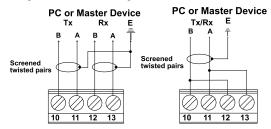
4-Wire & 2-Wire Communications Interface Connections
