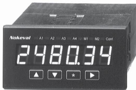
Panel meter 2021 is designed specially for temperature sensors and for common process inputs. 2021 base card has three card slots: One (slot A) for measuring card and two (slots B, C) for output and alarm cards.
