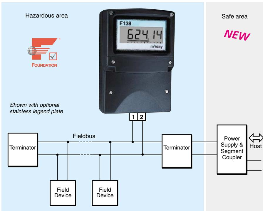
**The BA414DF Fieldbus Indicator** is a new cost-effective intrinsically safe field mounting instrument that displays a single fieldbus process variable in a hazardous area. Housed in a robust IP66 GRP enclosure, the instrument has a large, high contrast five digit display, plus a horizontal bargraph. The BA414DF indicator uses the same technology and compliments the well established BEKA eight variable fieldbus displays that are now in worldwide use.
