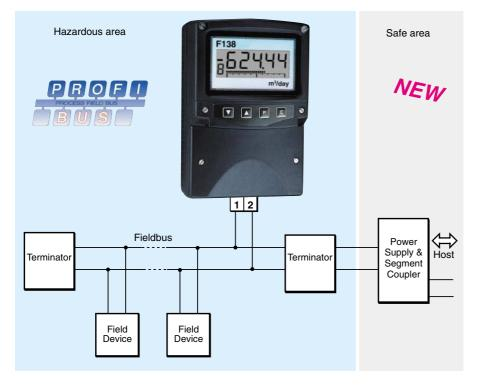
The BA444DF-P PROFIBUS Indicator is an intrinsically safe instrument that can display up to eight fieldbus process variables within a hazardous area. A numeric annunciator on the left hand side of the screen shows which variable is being displayed. This version of the indicator supports PROFIBUS PA protocol; for FOUNDATION™ fieldbus systems an alternative version is available − please see BA444DF-F FOUNDATION™ fieldbus datasheet.
