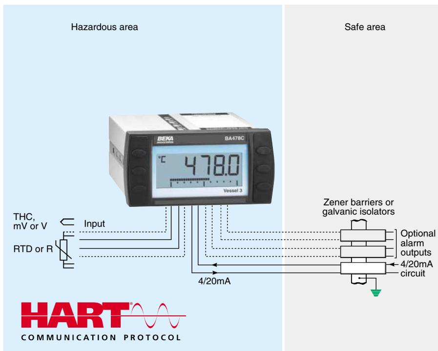
The new BA478C is a second generation panel mounting intrinsically safe loop powered indicating temperature transmitter which replaces the BA378C. It provides an accurate local digital temperature display, plus a 4/20mA output that may be scaled to represent any temperature range. Although incorporating new facilities such as HART® digital communication, diagnostics and a robust enclosure with an IP66 front, the BA478C remains electrically and mechanically compatible with the earlier model.
