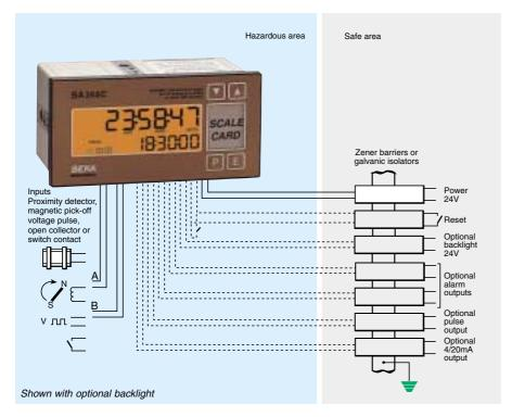
The BA368C is an intrinsically safe multi-function instrument which may be programmed to perform a host of counting and timing functions. Easy to use menus allow the instrument to be configured as a counter, timer, tachometer or as a clock. Both of the inputs will operate from 2-wire proximity detectors, switch contacts, magnetic pick-offs, open collector or voltage pulses. Optional alarm/control outputs further extend the many applications.
