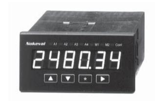
Counter 2061 suits well for distance measurement of various movement sensors, piece count or for dosage. Counter has red or green display, count up or down. Input pulse can be scaled to correspond desired number value, f.ex. one pulse may correspond three numbers or part of numbers in display (1 pulse=0.034 digits in display). Display memory (option) stores calculated value for one week after power brake.
