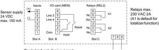
Card slot A only for input card. Slots B and C for optional cards.
