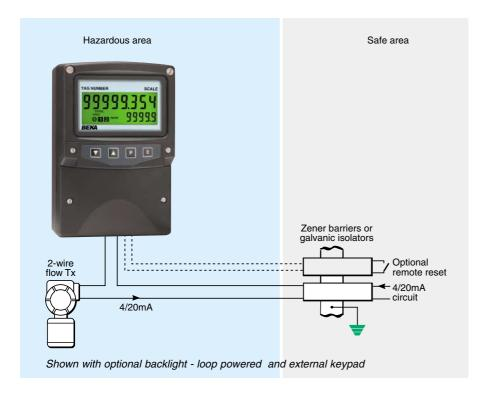
The BA354E loop powered 4/20mA rate totaliser is a third generation field mounting instrument that is electrically and mechanically compatible with the earlier BA354D, but it has a larger display, extended operating temperature and additional features such as a lineariser and bi-directional flow capabilities. Like its predecessor the BA354E is housed in a robust IP66 GRP enclosure with a separate terminal compartment.
