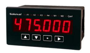
The panel meter 2251 is designed for two pulse sensors such as NPN-, PNP-, Namur -sensors, closing contact or pickup. The meter calculates the difference between the input frequencies, subtraction A-B, or alternatively, the meter divides the input frequencies, division A/B.
