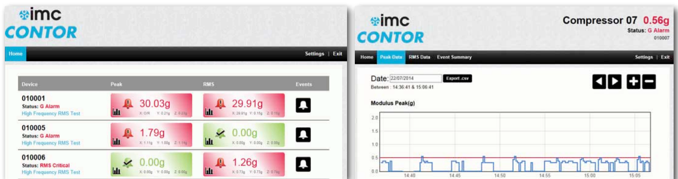
Above: Alarms appear in red and further analysis is available through the graph icons.
