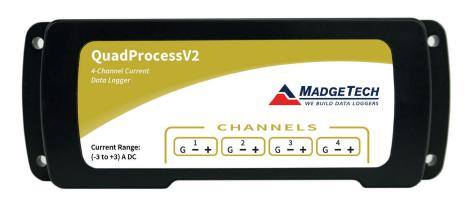
The QuadProcessV2 is an 4-channel, battery powered, low level DC current data logger with a reading rate of up to 4 Hz. It can measure and record 523,776 readings per channel. To maximize memory capacity, users can enable or disable channels. For easy identification, each channel can be named with up to a ten digit title.
