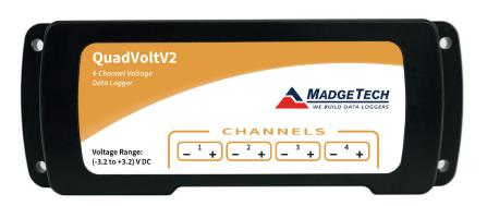
The QuadVoltV2 is an 4-channel, battery powered, DC voltage data logger with a reading rate of up to 4 Hz. It can measure and record 349,184 readings per channel. To maximize memory capacity, users can enable or disable channels. For easy identification, each channel can be named with up to a ten digit title.
