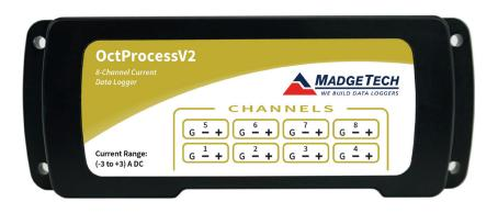
The OctProcessV2 is an 8-channel, battery powered, low level DC current data logger with a reading rate of up to 4 Hz. It can measure and record 261,888 readings per channel. To maximize memory capacity, users can enable or disable channels. For easy identification, each channel can be named with up to a ten digit title.
