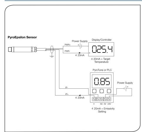
The PyroEpsilon Series is a range of high quality, low cost, compact sensors which measure the temperature of inaccessible or moving objects and materials. They measure temperatures from -20°C to 500°C, accurately and consistently, with an outstanding response time of 240 ms.
