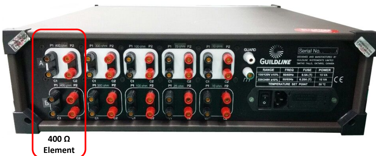
Model 7334-TC with 10 Custom Elements in a Temperature Controlled (TC) Enclosure
