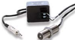
Remote Magnetic Sensor (MT-190-P) Gap 0.25 inches
