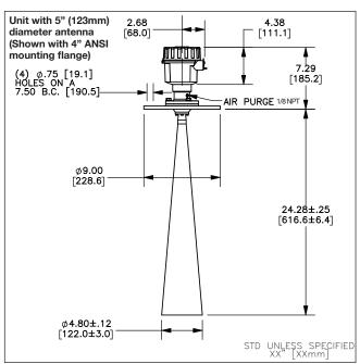
Dimensions shown represent units with or without dust shield-equipped antennas.
