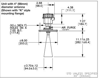
Dimensions shown represent units with or without dust shield-equipped antennas.
