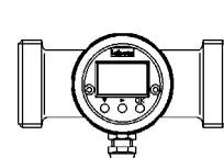
Standard position of display module and electrical connection.
