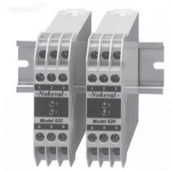
Our model 620S temperature transmitter is designed to meet the most exacting temperature measuring requirements. Extreme accuracy is obtained by linearizing the measurement signal with an accuracy of 0.05 % to the temperature. Thus one transmitter can now replace several of narrower range without reducing accuracy. Leadwire resistance automatic compensation up to 50
