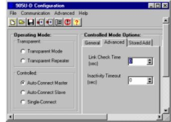
the master will transmit the check message up to five times. If there is still no ACK, then the master will reset the link (DCD reset).
