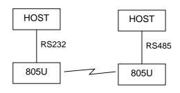
can connect to different types of serial signals. For example, RS232 data from one host device can be transmitted to a remote 805U unit and output as RS485 data to another host device.
