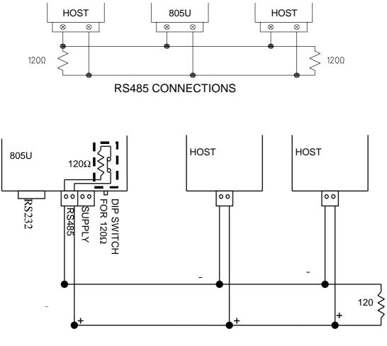
RS485 CONNECTION USING TERMINATING RESISTOR
