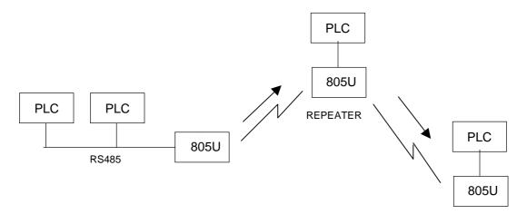
In controlled mode, up to five repeaters may be configured for any transmission path. The repeaters are configured by address.
