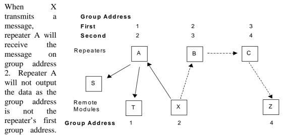
Repeater A will re-transmit on group address 1 to modules S and T. But repeater B will not accept the re-transmitted message on group address 1.
