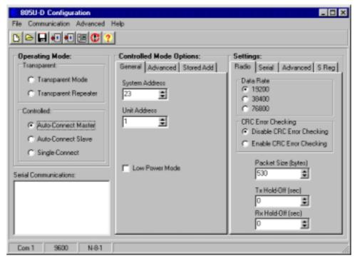
At the master unit, you need to enter the address of the slave. Select the "Stored Add" page and "Dest1". The address of the slave is entered into "Dest Add 1" and up to five repeater addresses may be entered. Repeater modules may be configured in any controlled mode option, but they must have the same system address. The repeater addresses are entered in order from the master - that is, "Rpt 1" is the first repeater after the master.
