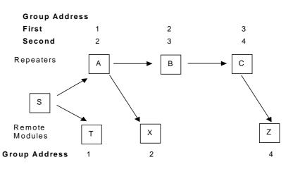
address as it is not configured as a repeater). When S transmits a message, T and A will receive it and output the data. If module X can hear the message, it will not output it as module X is configured with group address 2.
